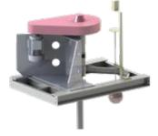
Fully automatic pulp level controller equipped with an ultrasonic sensor provides desired froth thickness precisely.
